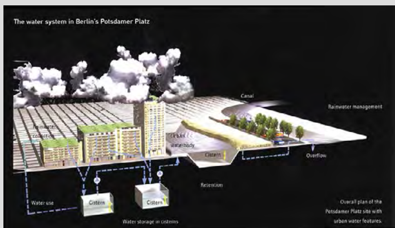
FIGURE 5-59 As shown to the left and below, stormwater is collected and stored on-site in a series of vaults. Water is circulated through a series of biofiltration areas and used for toilets and other mechanical systems in the building complex. Large storms overflow into an adjacent canal. SOURCE: Reprinted, with permission, from Herbert Dreiseitl, Dieter Grau (2001). Copyright 2001 by Birkhäuser Publishing Ltd.
