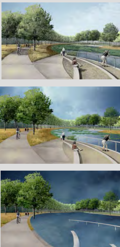
FIGURE 5-60 Illustrations show consolidated treatment areas in proposed parks. The top image illustrates the fair weather condition, the center image the water quality capture volume, and the bottom image the 100-year storm event. Construction was completed in spring 2007. SOURCE: Courtesy of Wenk Associates.
