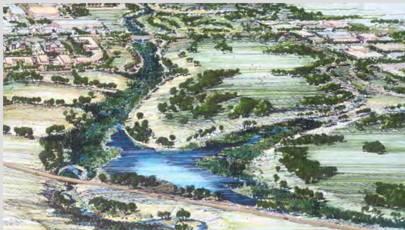
FIGURE 5-55 The community plan, shown on the left, is organized around two day lighted creeks, formerly buried under airport runways, and a series of secondary conveyances which provide recreational open space within neighborhoods. The image above illustrates one of the multi-functional creek corridors. Consolidated stormwater treatment areas and surface conveyances define more traditional park recreation and play areas. SOURCE: Courtesy of the Stapleton Redevelopment Foundation.
