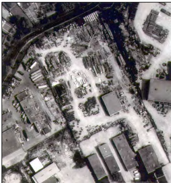
FIGURE 3-4 Example of a high-resolution panchromatic aerial photograph of an industrial area used for measurements of urban surfaces. SOURCE: Pitt and McLean (1986).
